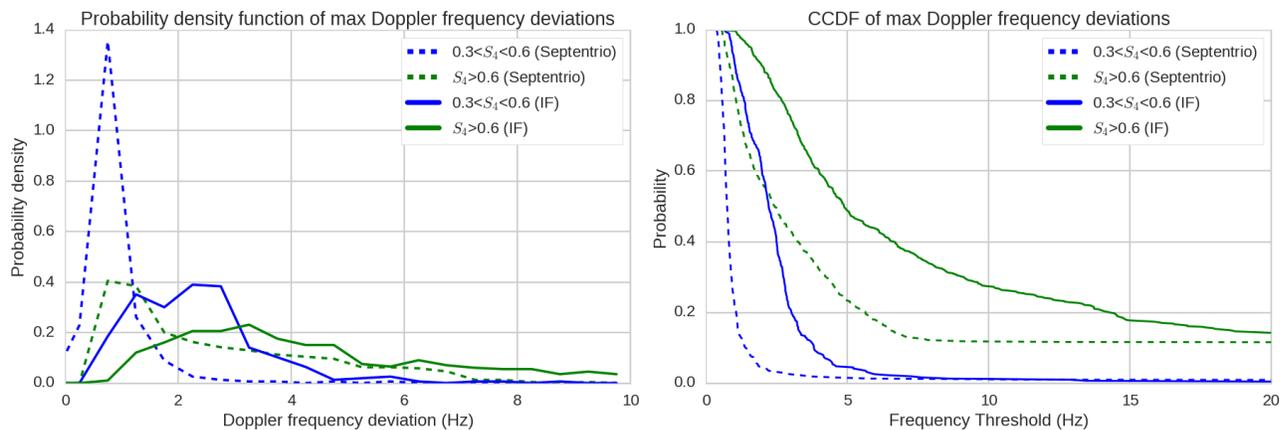
**Figure 2.** The PDF and CCDF distributions for the Ascension Island data. The distributions are generated by binning maximum Doppler frequency deviation values for the GPS L1CA signal.
