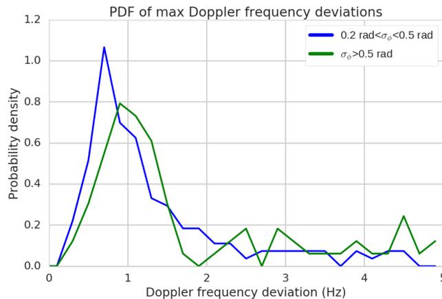
**Figure 3.** The PDF distributions for the Alaska data. The distribution is generated by binning maximum Doppler frequency deviation values for the GPS L1CA signal.
