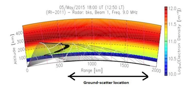
• It is a monostatic HF system operating at 8-18 MHz, that simulates a two way propagation link using ionospheric reflection.
